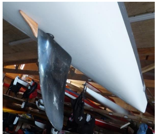
Sea kayak modified to have an underslung rudder. The wooden thing is a weed guard.
