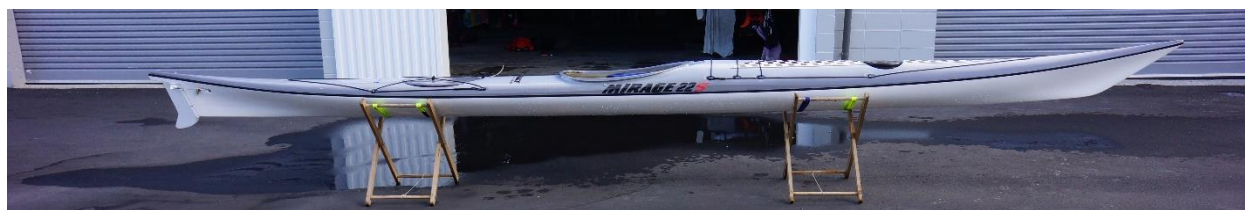
Mirage 22S racing sea kayak. Note extreme length and wacko rudder
