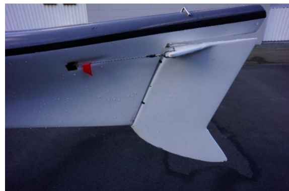
Mirage 22s with modified long rudder
