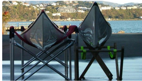
It's a skinny boat alright. Standard sea kayak 60 cm wide & Mirage 22s 45 cm wide
