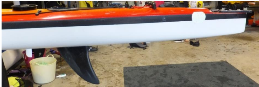
Underslung rudders steer brilliantly but are trouble on beaches
